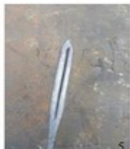
5 Forge a blunt taper on the end of the loop. Keep to the outer end as much as possible to avoid thinning the loop sides.
