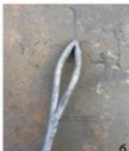
6 Begin spreading loop with a chisel. Avoid stressing the weld. Gripping weld with tongs while spreading can help if needed.
