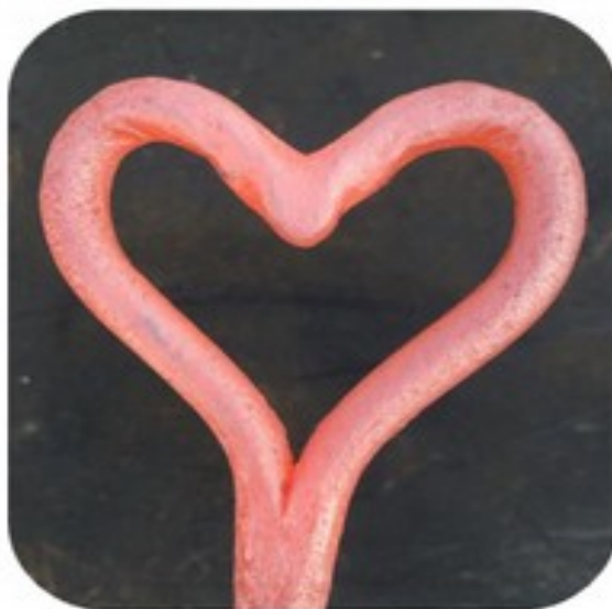
6 Begin spreading loop with a chisel. Avoid stressing the weld. Gripping weld with tongs while spreading can help if needed.
