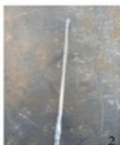
2 Upset an area at about 10" or 12" from the end. Then upset and scarf the end.
