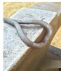
8 Bend outer 1/3 of loop on rounded edge of anvil then turn over and roll point in on anvil face until you have a flat heart shape. Fine tune curves on the horn as required.
