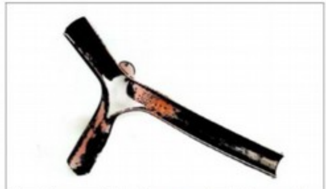
Partially opened 1/2-inch copper pipe. Take care that the opening in the middle remains symmetrical.
