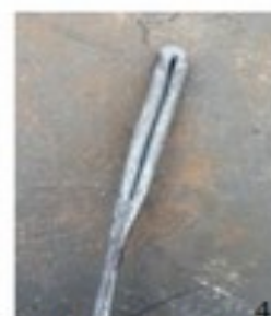
4 Forge weld joint and then flatten out the remaining loop.
