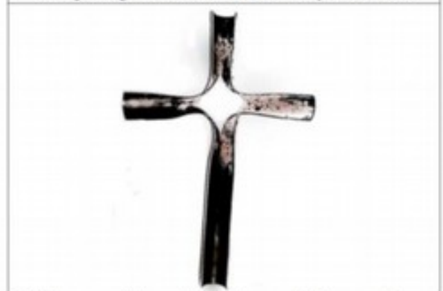
Fully opened piece, but the four ends have not been rolled closed to form 1/4-inch pipe.
