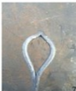
7 Continue spreading on the anvil horn. Spread the outer end most.
