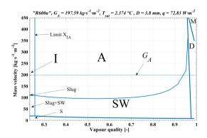
Figure 7. Flow pattern map for test B for the R600a refrigerant with  $T_{\rm sat}=2,374$  °C, D = 3,8 mm, q = 72,83  $W{\cdot}m^{-2}$  and  $G_A=197,59~kg{\cdot}m^{-2}{\cdot}s^{-1}$
