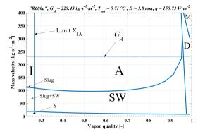
Figure 6. Flow pattern map for test B for the R600a refrigerant with  $T_{sat} = 5.71$  °C, D = 3.8 mm, q = 155.73 W·m<sup>-2</sup> and  $G_A = 229.43$  kg·m<sup>-2</sup>·s<sup>-1</sup>
