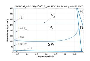
Figure 4. Flow pattern map for test B for the R600a refrigerant with  $T_{sat} = 11,63$  °C, D = 3,8 mm, q = 488,27 W·m<sup>-2</sup> and  $G_A = 267,26 \text{ kg}\cdot\text{m}^{-2}\cdot\text{s}^{-1}$
