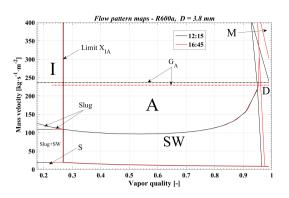
Figure 9. Comparison of the maps corresponding to tests A and D at 12:15 and 16:45, respectively
