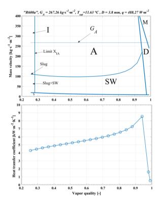
Figure 13. Contrasting of flow pattern maps vs. heat transfer coefficient for the Wojtan *et al.* [8], [28] mathematical model
