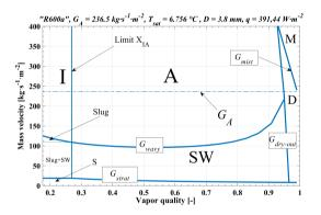
Figure 3. Flow pattern map for test A for the R600a refrigerant with  $T_{sat} = 6,756$  °C, D = 3,8 mm, q = 391,44 W·m<sup>-2</sup> and  $G_A = 236,5$  kg·m<sup>-2</sup>·s<sup>-1</sup>
