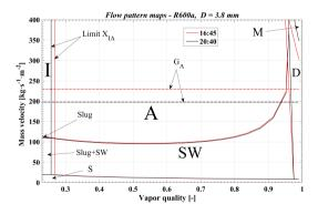
Figure 10. Comparison of the maps corresponding to tests D and E at 16:45 and 20:40, respectively
