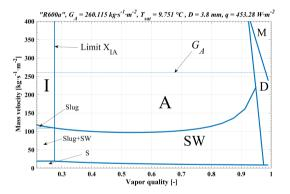
Figure 5. Flow pattern map for test B for the R600a refrigerant with  $T_{sat} = 9,751$  °C, D = 3,8 mm, q = 453,28 W·m<sup>-2</sup> and G<sub>A</sub> = 260,115 kg·m<sup>-2</sup>·s<sup>-1</sup>
