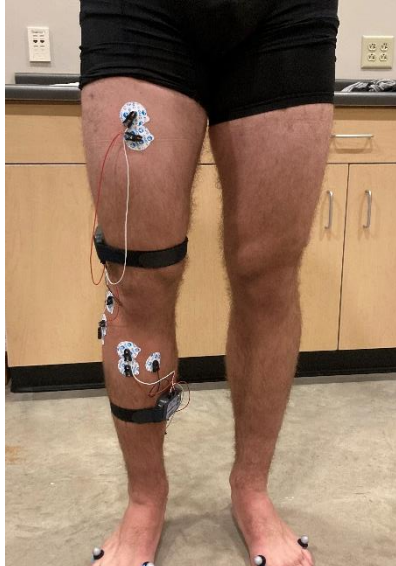
Figure 4: EMG Setup- Frontal Plane
