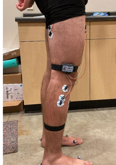
Figure 5: EMG Setup- Sagittal Plane
