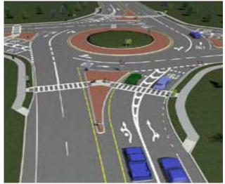
Vehicles should be directed into the proper circulatory lane at the approach entrance (yield) line. Lane lines should be designed tangential to the roundabout, as shown in KRG Exhibit 6-21.
