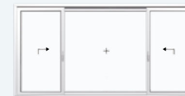
System K 2 lift/sliding sashes, 1 fixed pane
