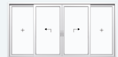
System C 2 lift/sliding sashes, 2 fixed panes
