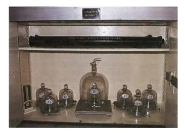
Fig. 1 The International prototype of the kilogram and its six designated copies which are kept at the Bureau International des Poids et Mesures at Sèvres
