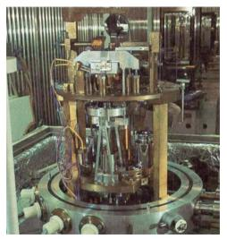
Fig. 5 The NBS-2 balance at BIPM, with which 1 kg mass standards can be compared to better than 1 part in 10<sup>9</sup>. This balance was made at NBS and presented to BIPM in 1970
