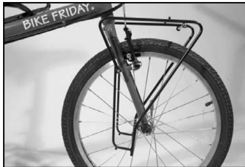
Fig. 6 Completed front rack.
