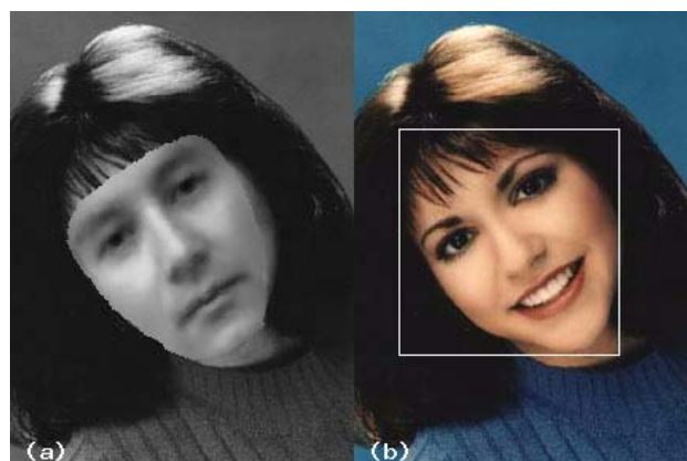
Figure 4. (a) Best-match pose of the model face shown in Fig. 3b in the luminance component of color image shown in Fig. 2a. (b) Detected face is enclosed in a square. The center of the square is at the tip of the nose of the model face when matching the luminance image.
