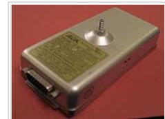
A typical altitude encoder, the ACK Technologies A-30. Note the 15-way D-type connector to send the Gillham code to the transponder and the port on the top of the case that connects to the aircraft's static pressure system.
