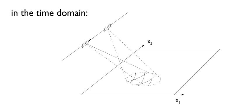
Each view gives slices of the ground reflectivity function Reconstruct a function from its integrals over lines use FBP
