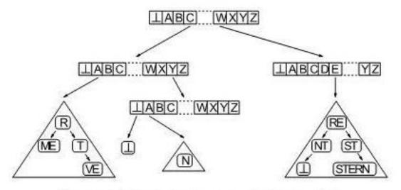
Figure 2: Burst trie after insertion of a record with key "western".
