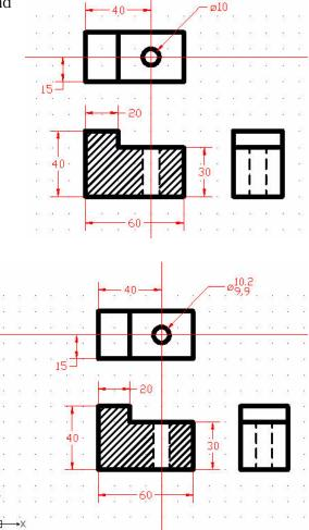
Apply a Tolerance to the diameter dimension to complete the drawing.
