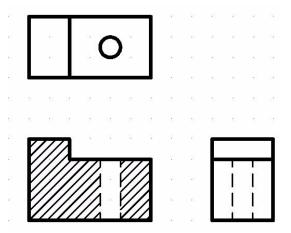
In normal drafting practice, the Hidden Lines need to be converted to an Object Line for this setion view. This is only an example of the command available.
