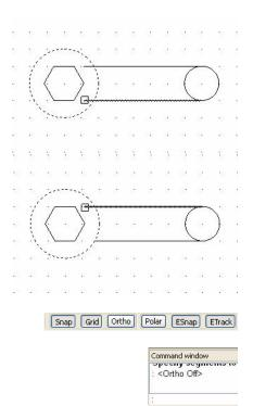
filleted entities do not have to intersect, and they can overlap. If the entities overlap, they will be trimmed (by default) to create the rounded corner. In any case, the Lines to be filleted are connected to the fillet arc.
