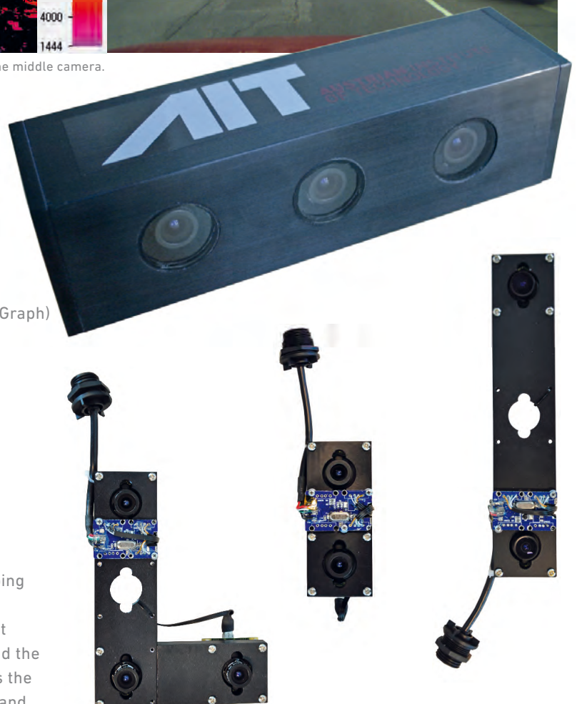
Fig. 4: Different stereo camera configurations.
