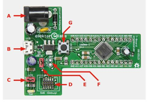
This T-Board is a perfect platform for an ARM Cortex-M0+ microcontroller ID, is by default not connected to the MCU (in order to free up available pins). A solder jumper however allows you to connect it to pin PA03. The ID pin is used for USB On the Go (OTG); refer to Atmel's application note for more details [1].
