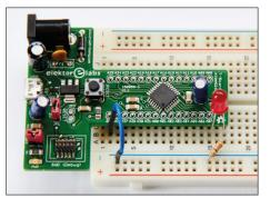
Figure 3. This ARMed-T-Board-on-a-breadboard is all ready to go.
