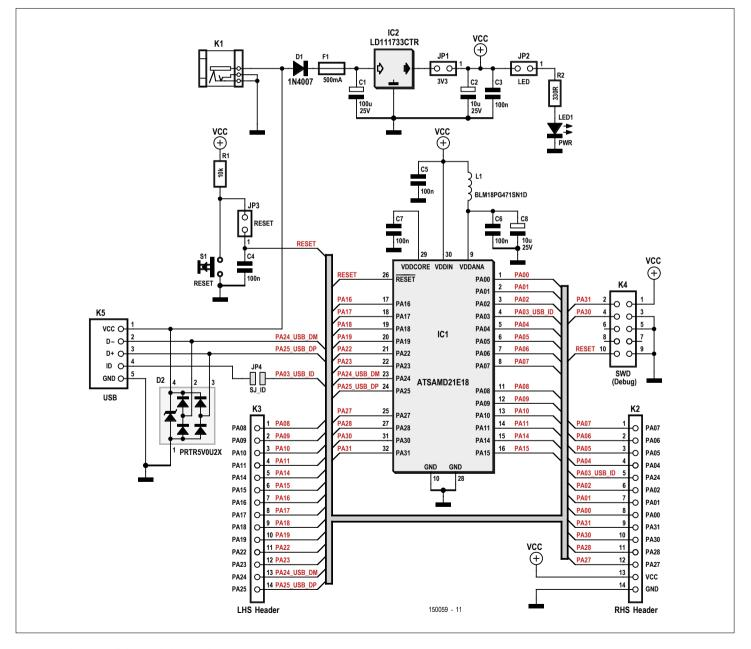
Figure 1. Schematic of the ARM'ed T-Board.
