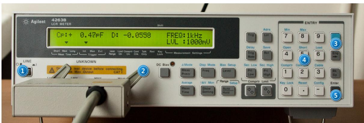
Picture 2. View of the RLC bridge front panel: 1 – switch; 2 - wire terminal; 3 – additional function button; 4 – SHORT button; 5 – ENTER button.
