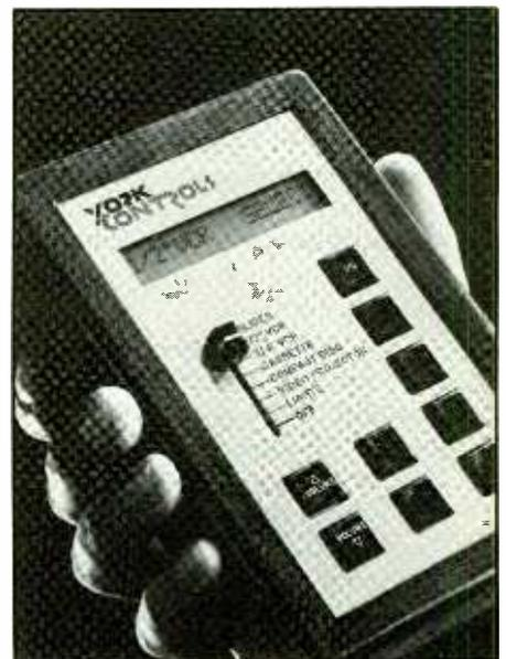
capable of controlling up to 72 functions of a York Control System, commanding any combination of home-entertainment or/and environment equipment. Up to eight different pieces of equipment can be selected using a slide switch mounted on the faceplate. Up to nine pushbuttons can also be mounted on the faceplate to give the TD-72 a maximum 72-function capability.
