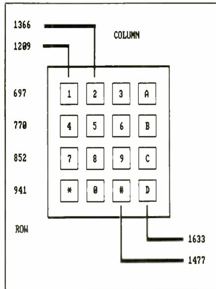
Fig. 2. A tone-type DTMF dialing keypad can have a total of 16 keys, though all but the ones labeled "A" through "D" are normally found on current home and business telephone instruments.
