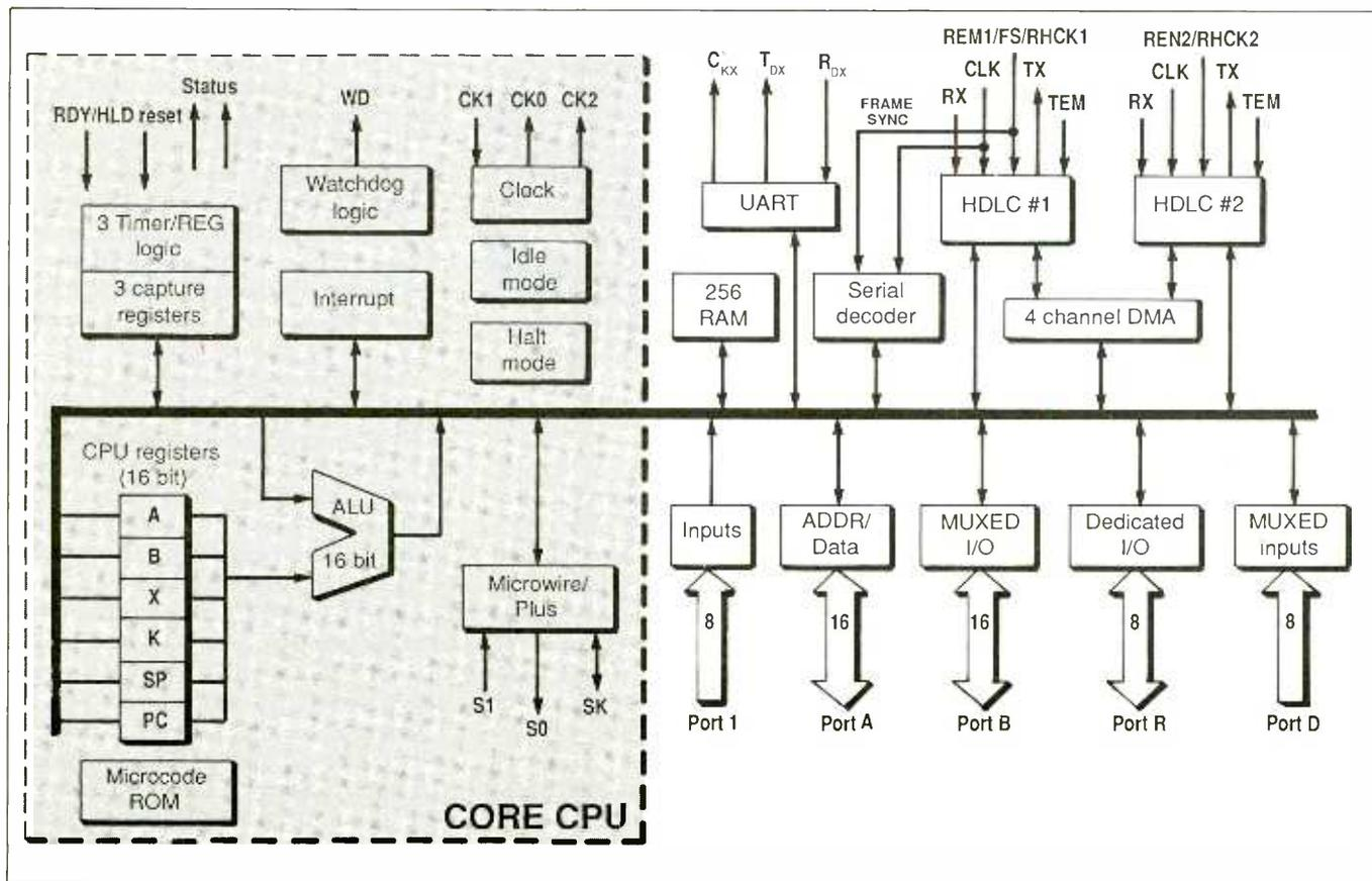
Fig. 1. National Semiconductor's 16-bit HPC16400 High-Performance microController has a common core CPU and unique memory and I/O configurations suitable for specific applications.
