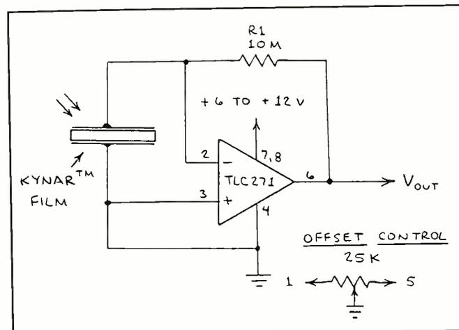
Fig. 7. A high-impedance amplifier for Kynar™ pyroelectric film.
