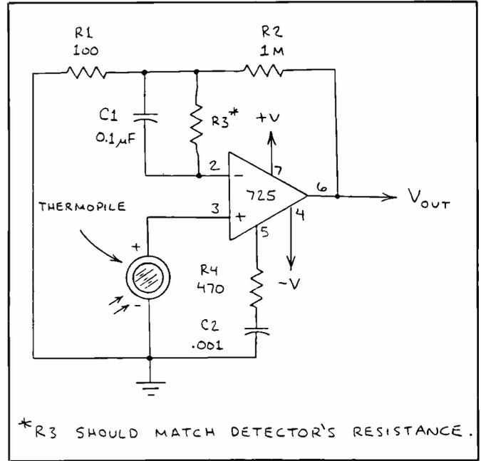
Fig. 5. A precision amplifier for a miniature thermopile.
