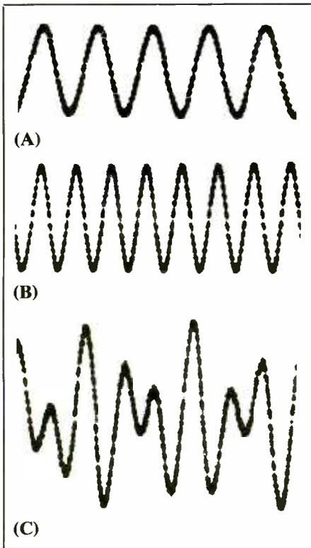
Fig. 1. Examples of DTMF tones generated when (A) a Row 3 button is pressed on the dialing keypad (582 Hz); (B) a Column 2 button is pressed (1,336 Hz); and (C) the "8" button is pressed (algebraic sum of Row 3 and Column 2 signals).
