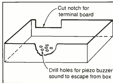
Fig. 4. Machining details for the project's enclosure.
