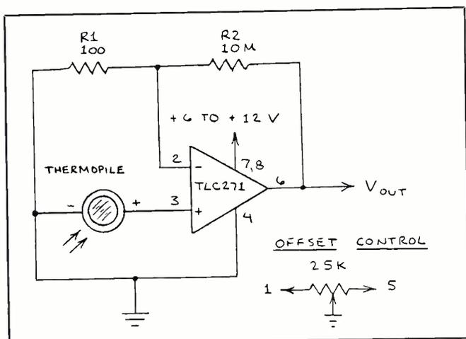
Fig. 6. A low-power amplifier for a miniature thermopile.
