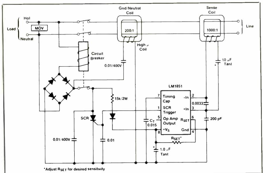
Fig. 5. A typical ground fault interrupter circuit.
