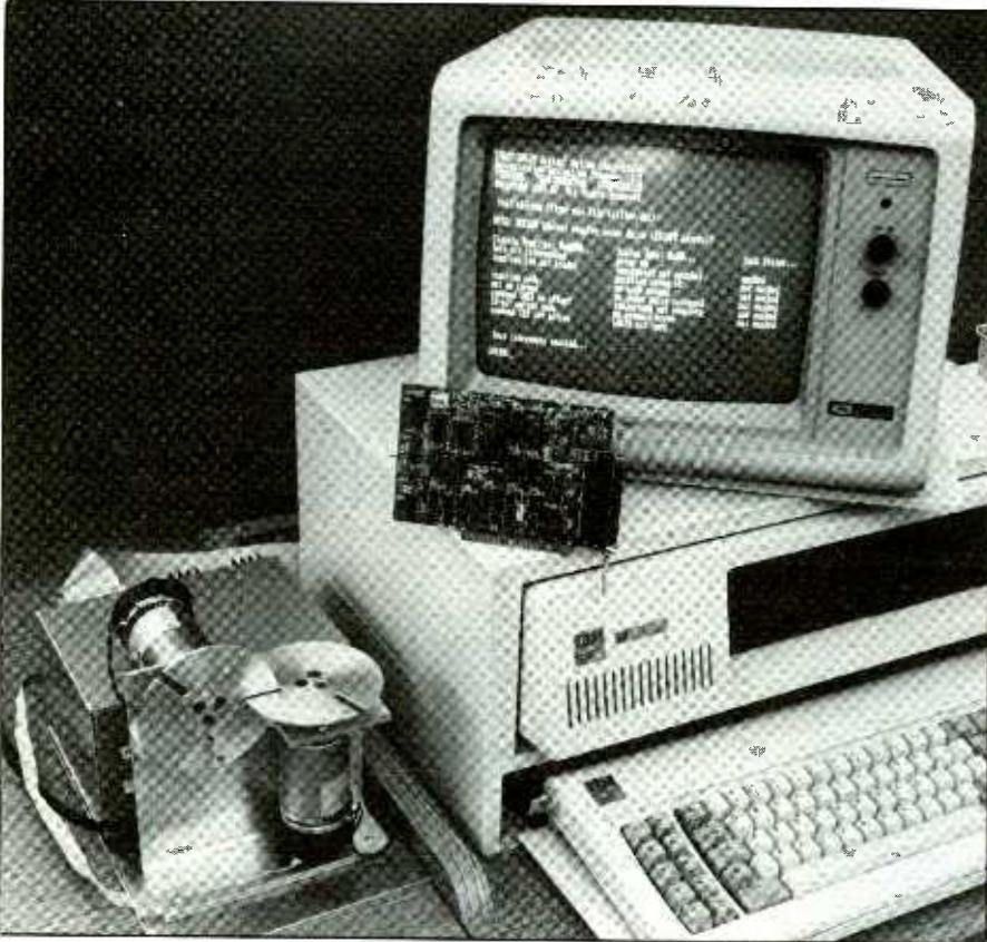
*Fig. 2. The LM628 motion-control processor governs the position, velocity and acceleration, rates of servo mechanisms. The LM628 evaluation board is shown in front of the video monitor in this photo.*
