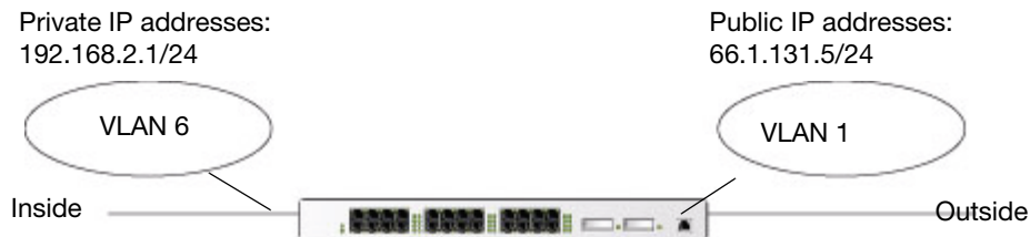
Figure 3 Example: Source NAT using Controller IP Address
