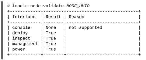
Replace *NODE\_UUID* with the unique identifier for the node. Alternatively, use the node's logical name. The output of the command above should report either **True** or **None** for each interface. Interfaces marked **None** are those that you have not configured, or those that are not supported for your driver.
