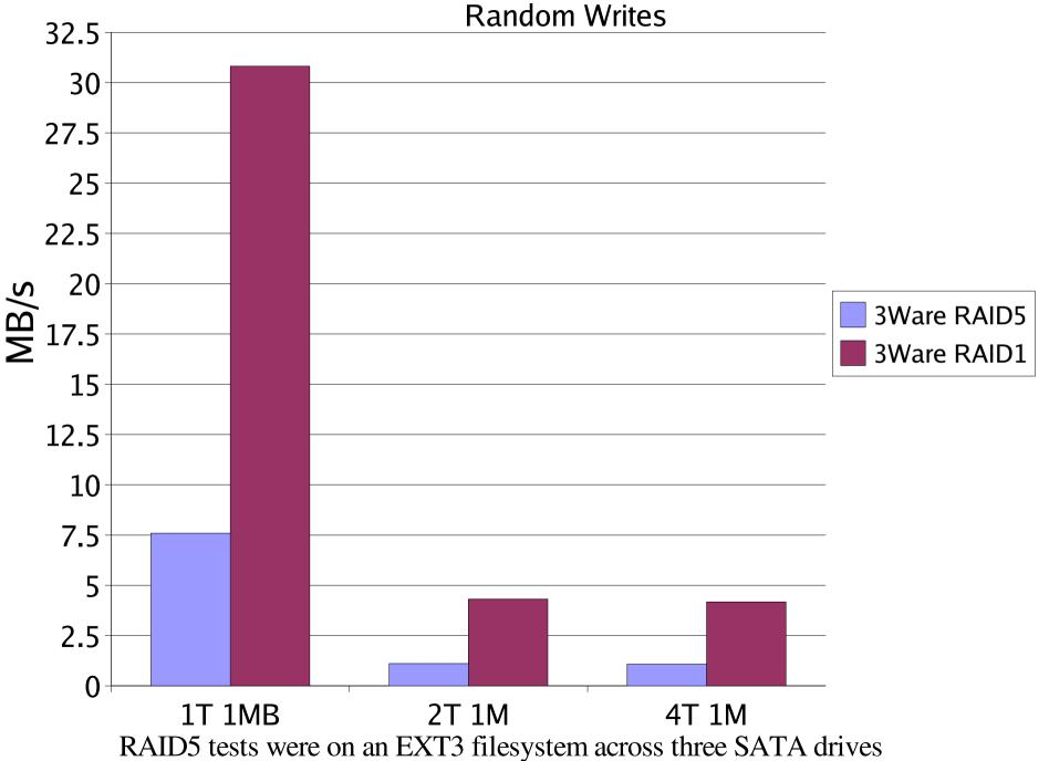
RAID5 tests were on an EXT3 filesystem across three SATA drives RAID1 tests were on an EXT3 filesystem across two SATA drives
