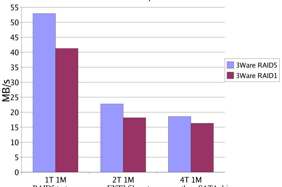
RAID5 tests were on an EXT3 filesystem across three SATA drives RAID1 tests were on an EXT3 filesystem across two SATA drives
