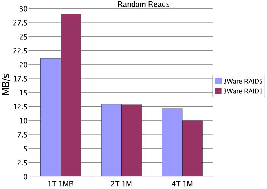
RAID5 tests were on an EXT3 filesystem across three SATA drives RAID1 tests were on an EXT3 filesystem across two SATA drives
