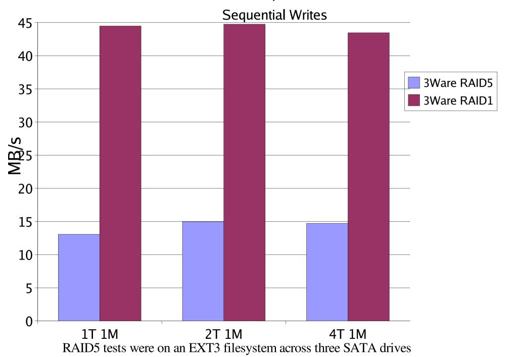
RAID1 tests were on an EXT3 filesystem across two SATA drives
