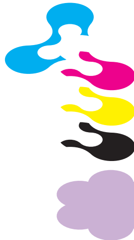
Difference blending mode produces five color plates: flattening requires conversion of spot into process colors to properly blend the colors.
