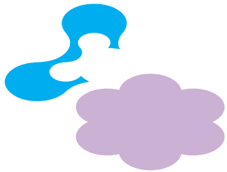
No transparency effects produces two separation plates: for cyan and Pantone 530 object.
