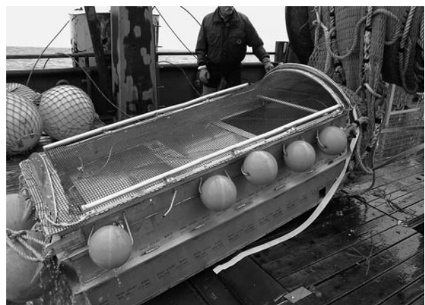
Figure 1. Aquarium codend (livebox) ascending the stern ramp of the vessel Medeia . A trap door in the stern of the aquarium codend allows fish and invertebrates to enter a water-filled chamber free of turbulence.
