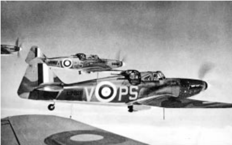
Defiant 2 seat fighter formation. These aircraft were designed with a rear turret but no forward firing guns.
