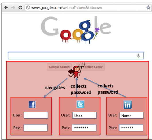
Figure 2: Lupin arranges the injected frames in a hierarchical fashion. Each target web page is loaded asynchronously.
