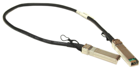
Figure 9: SFP+ DAC cable
