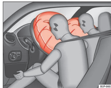
Fig. 19 Inflated front airbags
