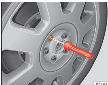
Fig. 158 Changing the wheel: hexagonal socket in screwdriver handle to turn the wheel bolts after they have been loosened
