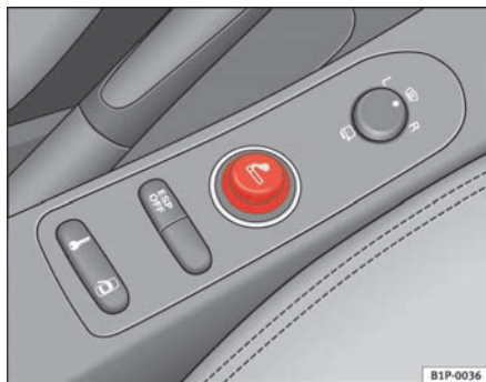
Fig. 100 The cigarette lighter is located in the electric socket on the front of the centre console
