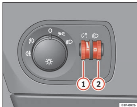
Fig. 74 Instrument panel: regulation for instrument and switch illumination and headlight range control
