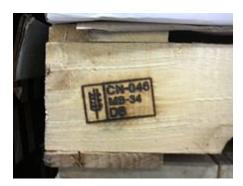
ISPM 15 markings on a pallet from China. The **MB** indicates the wood has been fumigated with methyl bromide to kill pests.
