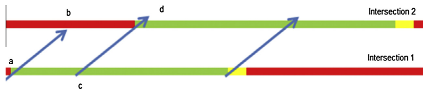
Fig. 15. Time space diagram of link 2 at PM.
