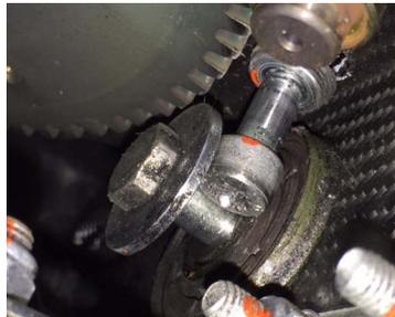
11. Raise motor (taking care not to snag or crush loose wires and hoses).
