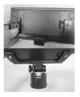
Install the **Support Part 2** on to the bracket that is a part of the PT253. Make sure the **Spacing Tube** is inserted over the locking screw and between the arms of the bracket. Install the Allen screws to **Support Part 2**, it can now be fitted over a round a pole 38mm in diameter and locked in place with the Allen screws, or continue to the next step for mounting to a flat surface.
