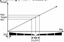
Check weighing operation first requires the nominal weight and tolerance values to be entered in to the PLU memory.
