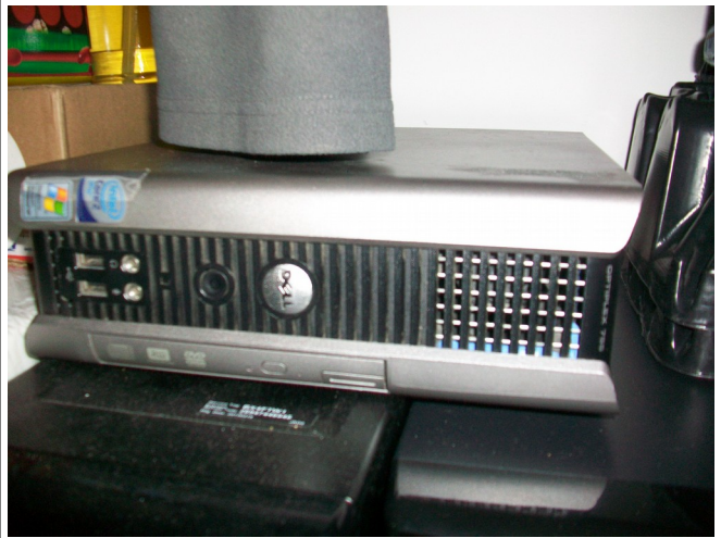
Dell Optiplex 755 USFF. Intel Graphics media accelerator 3100. 2GB RAM. Processeur Duo 2.8 Ghz.
