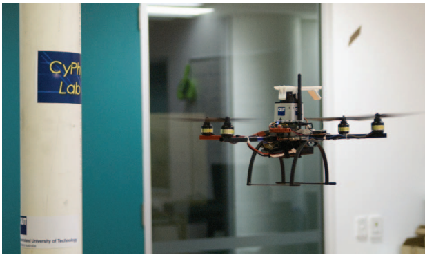
Figure 15. Mikrokopter-based quadrotor equipped with Gumstix and LRF [32].
