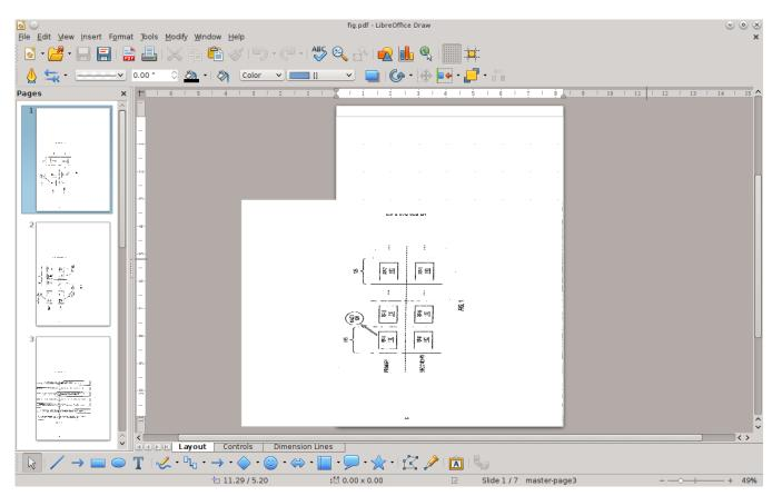
2) File opened in LibreOffice Draw: page size is correct, but the contents (figure) is deformed. The right bottom corner is in correct position, width and height are swapped.
