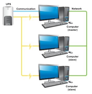
One UPS, multiple computers. Only one of them can actually talk to the UPS directly. That's where the network comes in. The Master system runs the driver, upsd, and upsmon in master mode. The Slave systems only run upsmon in slave mode.
