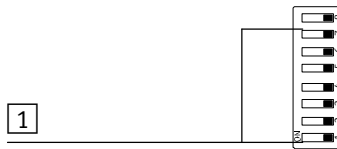
Fig. 1/4: Setting the station number (8-element DIL switch 3)
