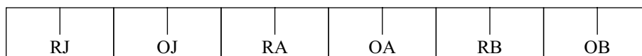
Figure L-17 — Organization of the contents of the EP field for the CIEJab (EnumCS = 19)
