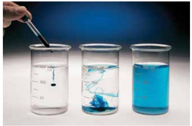
Figure 3.9 An example of diffusion. As a drop of ink gradually dissolves in a beaker of water, the ink molecules diffuse from the region of their higher concentration to a region of their lower concentration. APR
