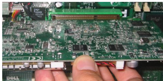
Align the card with the AGP slot
