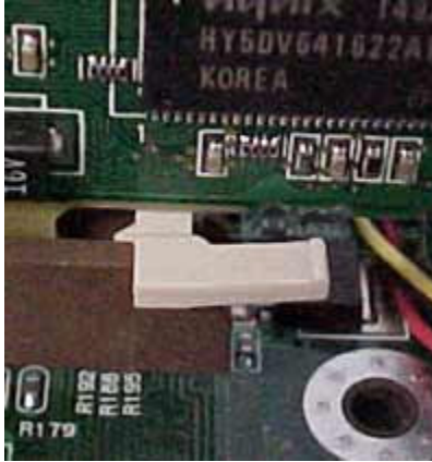
Example of an AGP lock (locked position)
